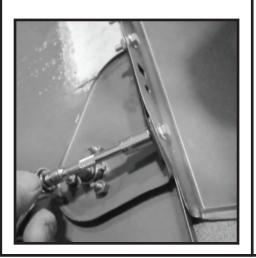
6 - Installation of fender is the reversal of steps (1)-(21) of the snorkel instructions. Reinstall windshield bracket. If windshield bracket does not line up correctly. Floating nut Plates in a-pillar can be broken free with a screwdriver to allow for additional movement.
