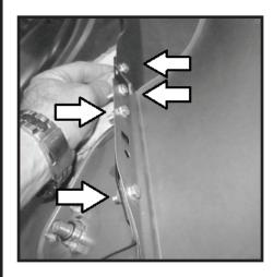
4 - Cowl should be aligned with outer edge of fender. Fender can be placed onto body to double check cowl placement (front to back). The left side fender can be used as a guide if needed.
