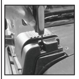
91 - With Low Mount Air Intake secure pull outer edge of "U" gasket away from Low Mount Air Intake until "U" Gasket rest flat against side of intake. **92** - Tighten all (6) caps head bolts.
