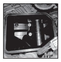
**49**- If Air Box does not fit within 1/8" (3mm) of rubber grommets the top of the silicone 90deg Elbow will need to be trimmed. Remove Air Box and 90deg Elbow. If Air Box fits correctly proceed to step (51).
