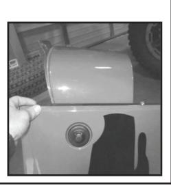
5 - Tighten M6 x 20mm Flange Hex Head Bolt and M6 Flange Nuts before reinstalling fender on vehicle. When fender is being installed remember to connect antenna cable.
