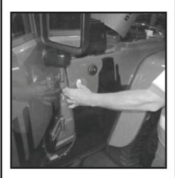
**3** - Align Cowl Re-mount Bracket to the holes of upper fender cowl plate and fender. Plate will be placed under fender as shown.
