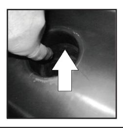
55 - Apply a thin film of sealant around end of Air Tube. An excessive amount may cause the elbow to slide off air tube when tightened. **56** - Apply sealant to the inside of two lower rubber grommets as shown. Make sure sealant completely fills the two holes.
