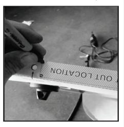
29 - With guide holes marked and guide holes drawn drill 1/8" centering holes into fender. Use a 7/32" drill bit to enlarge 1/8" guide holes. NOTICE: A wood block should be placed under marked hole as described in steps 23&24. Wood block will protect the fender if drill bit grabs panel.
