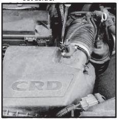
**41**- Remove factory air filter and set to the side. Filter can be reused if clean. A high flow after-market air filter can also be used with XHD diesel snorkel system.
