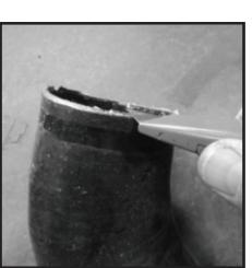
**51** - With Air Box in the correct location, 90deg Elbow attached to lower Air Box inlet and aligned with the Air Tube. Carefully remove Air Box and 90deg Elbow together. Mark the position of the 90deg Elbow to Air Box as shown. remove elbow for step (52).
