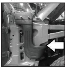
73- Inspect Cowl "Z"-Bracket to Main Body alignment.
