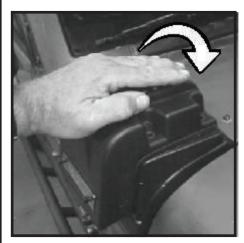
**90** - Using (4) M6 Short Caps Head Bolts and (4) M6 Flat Washers secure intake to Main Body.
