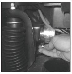
**47**- Place 90deg Elbow onto Air Tube. DO NOT install Hose Clamp. A test fit of Air Box will be required. 90deg Elbow will be removed and adjustments made prior to final assemble.
