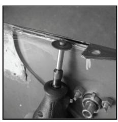
**33** - After cooling remove cut metal from fender. Care should be taken when handling rough cut metal. Removal of inner section will allow gasket to rest flush with fender.
