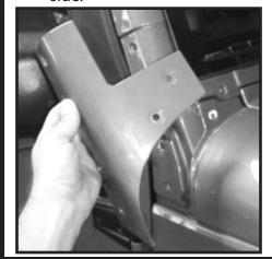
**3** - Remove the (4) cowl screws. A T-30 Screw driver or socket will be required.
