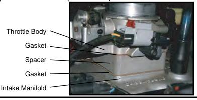
5. Remove 2 bolts that hold the throttle cable bracket to the intake manifold. Use supplied M6 Throttle Linkage Bolts and Throttle Linkage Spacers to space throttle cable bracket up. Re-Install intake tube.
