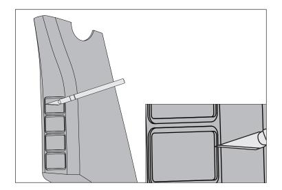
6. Insert switch into opening, cutting material as needed for a tight fit.
