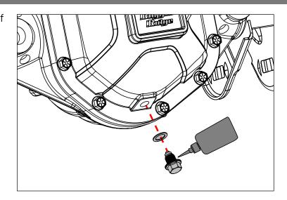
5. Install Dipstick Bolt and 1/4" Washer. Fill housing with gear oil. Periodically remove and check dipstick bolt for correct capacity. This will be indicated by oil on the Dipstick Bolt in the highlighted area. Do not fill past cross hatching marks. Ensure Dipstick Bolt is reinstalled after final check of full capacity.
