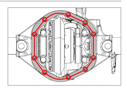
3. Install Boulder Differential Cover using supplied 5/16" Flange Bolts. Torque bolts to 30 ft-lbs using a criss-cross pattern.
