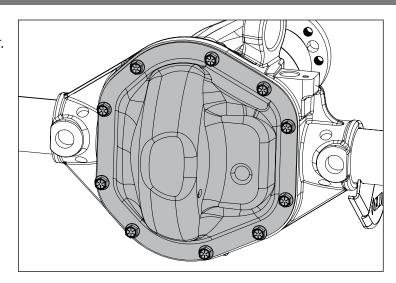
2. Apply RTV sealant to housing flange.
