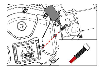
6. Install Fill Plug and 1/2" Washer.
