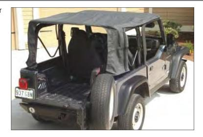
10. Ensure center bow is centered in hook and loop flap but DO NOT fasten at this time. Pull down and insert rear corners of soft top into belt rail. Secure header to windshield frame at this point.
