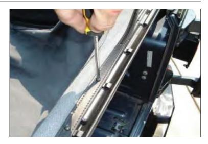
8. Wrap fabric over header and drape it over tailgate. Raise header slightly and work pockets in fabric over corners of header. Install screws removed in step 5 in corners of header.
