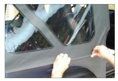
17. Install tailgate bar in receiver on each side of tailgate opening and insert rear window into "C" channel of tailgate bar.
