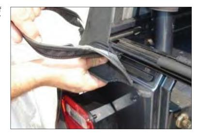
18. Start zipper of rear window. Hold up window and finish zipping rear window to top. Ensure tailgate bar is centered and securely fastened. Tuck flaps on rear window under soft top fabric.
