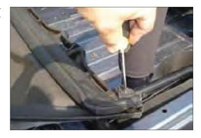
6. Flip top fabric into rear of vehicle so fabric lays bottom side up. Remove screws that fasten soft top fabric to windshield header and set aside for later use. Remove soft top fabric.
