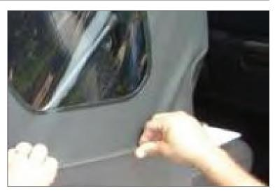
14. Push inner spreader bars up until they snap into place.
