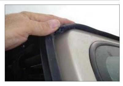
6. Lay fabric top over frame and orient it on vehicle. Snap fabric to middle and rear bows.
