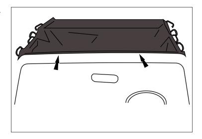
5. Attach the windshield header to the windshield using the bolt and curved washer provided.
