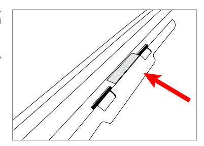
5. In an alternating pattern secure Sun Shade by looping straps around sport bar. DO NOT fully tighten at this time. Once all straps are secure, repeat pattern and pull tight.
