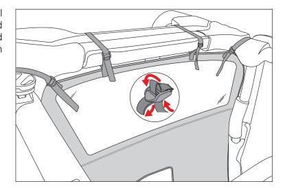
3. Secure windbreaker to seat brackets. Pull down gently on the gabric and thread straps through back of seat brackets. Buckle straps and tighten all straps.
