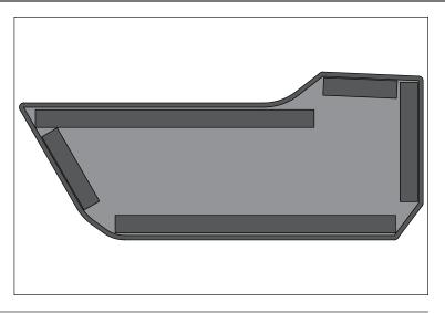
2. Clean lower area of door panel with isopropyl alcohol and apply adhesion promoter where hook and loop strips will tape to door. Allow 90 seconds for adhesion promoter to properly dry before continuing.
