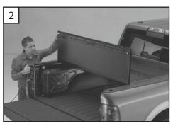
1 & 2. To open the cover: Lower the tailgate and pull the cable. While pulling on the cable lift the panel up and towards the cab, repeat for the next panel.
