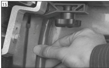
14. Attach the prop rod to the side rail.
