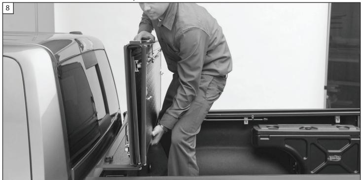
8. Place the tonneau onto the mounting rails with the smallest panel towards the cab of the truck and with the front flap covering the bulkhead.
