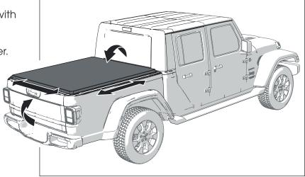
9. NOTE: When opening the cover, be sure to stow the tail clamps into the cover bow to prevent damage to the tarp when folded.
