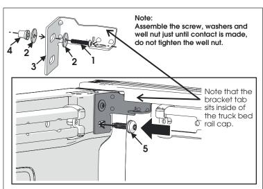
Use the well nut as a guide to insert the cab bracket into the bulkhead wall. Thread the cab bracket bolt (5) through the bracket and into the bulkhead. Snug the well nut, tighten the bolt to 17.5 N-m (155 in-lb).
