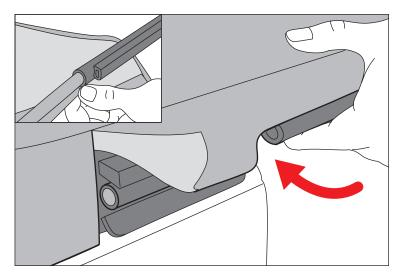
6. Roll plastic strip over edge and into side groove of body tub. Repeat for opposide side.
