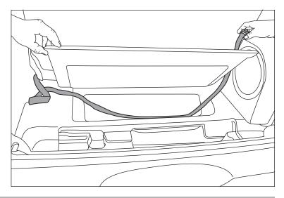
3. Fold back seat down and thread end of seat strap through child seat restraints. Thread strap through buckle and tighten as shown.
