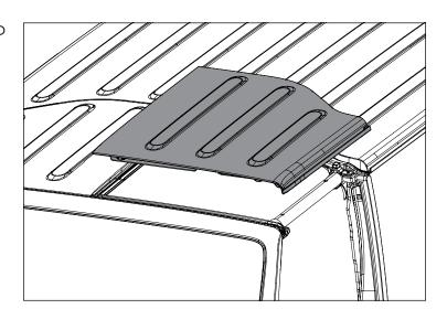
3. Install Pin Catch and Flat Washer inside of hole for hardtop screws. Place Oversized Flat Washer over Button Head Bolt and screw into Pin Catch. Button Head Bolt goes through fixed nut for hardtop bolt.
