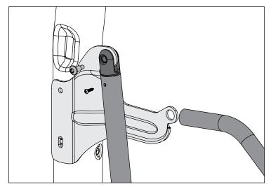
2. Insert Quick Release Bow Knuckles in open ends of soft top bows.
