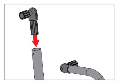
3. Pull quick release knob and turn clockwise to lock in open position.
