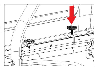
2. Remove freedom panels and remove two remaining hardtop screws using T-40 Torx driver.
