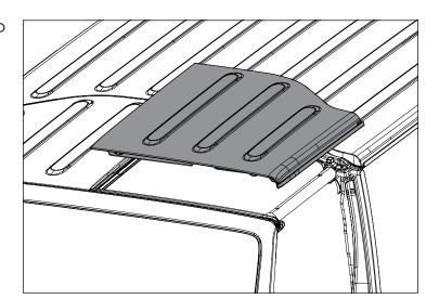
3. Install Pin Catch and Flat Washer inside of hole for hardtop screws. Place Oversized Flat Washer over Button Head Bolt and screw into Pin Catch. Button Head Bolt goes through fixed nut for hardtop bolt.
