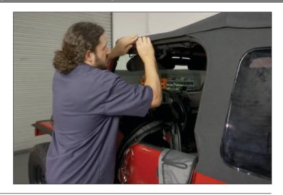
38. Slide rear window into rear tailgate bar. You'll notice a roll that slides into the channel of the tailgate bar.
