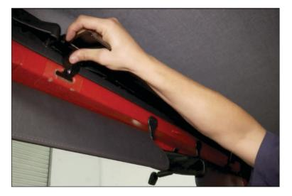
33. Move to the back of the Jeep and pull the sail panels down and flip the plastic guides into the body of the Jeep.
