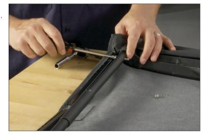
15. Now attach the center support bow to the side bows. This attaches just behind the hinge of the side bow. It requires a bolt and plastic washers. The plastic washers are used because this area will hinge when folding the top back. So when you tighten the bolt do not completely tighten it all the way allow for some play for the item to hinge. Just snug and test if the item can freely move.
