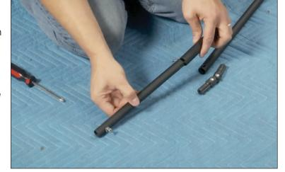
12. Now insert the hinge into the tube and fasten items with a screw. Slide the other end of the hinge into the larger "Dog Leg" tube frame piece. Align the predrilled holes and fasten with screw.
