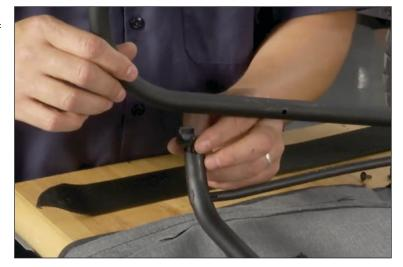
17. Attach the center bow strap to the center bow. The first screw will go through the strap into the center bow and into the plastic support piece. There are an additional two screws that go through the strap to the center bow.
