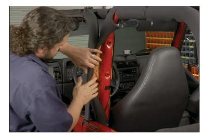
21. Each bracket should be stamped L (drivers side) and R (passenger side). The shallow pivot point is towards the top and the larger pivot point towards the bottom. Attach to the threaded inserts of the roll bar with two T-30 torque screws.
