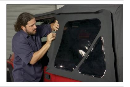
36. Insert lower plastic guide into the Jeep tub rail. Then meet touch fasteners surface of the window to the top.
