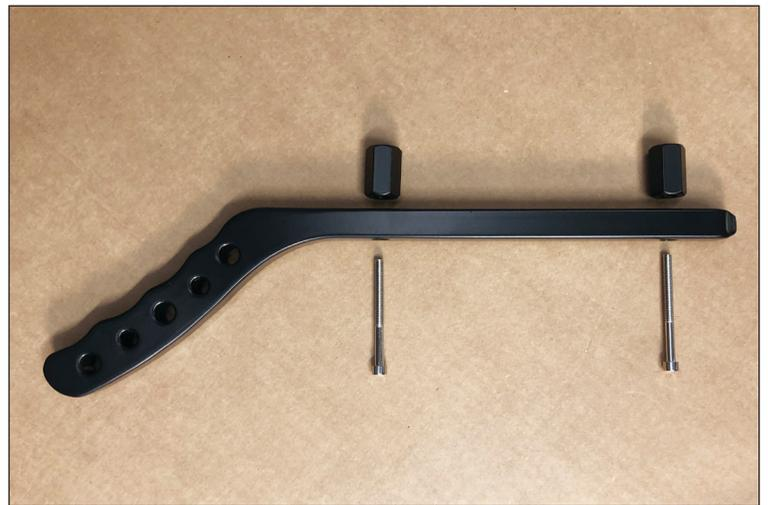
3. Insert Allen head bolt through the handle and then through the hex spacer into roll bar. **DO NOT** Overtighten the bolts or use power tools to tighten, it could cause the threads to be striped or bolt to break. When tightening alternate between to the two Allen head bolts to assure the handle seats flat to the roll bar.
