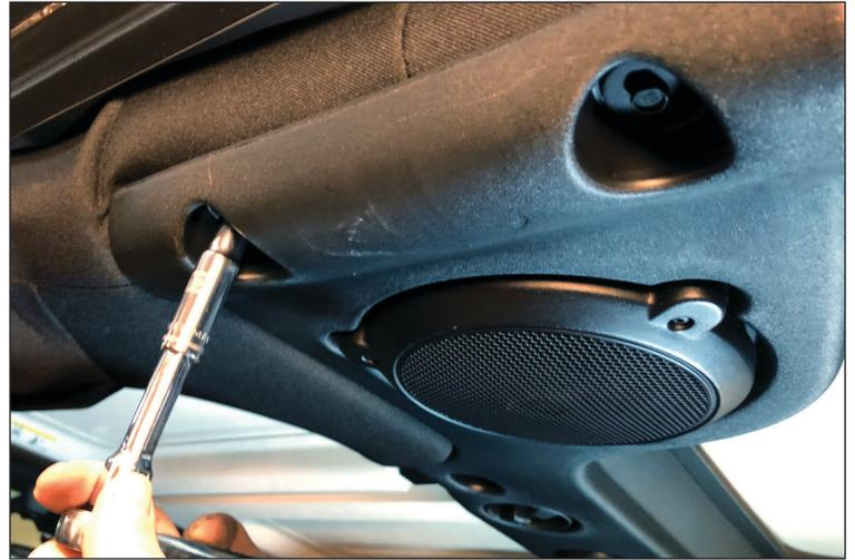
2. Now get the handle and hardware. The kit provides new longer Allen head bolts and hex spacers. Before installing simply thread Allen head bolts in the roll bar to assure threads are clean and free of paint, dirt or burs. Unthread the bolts and now install with the handle.
