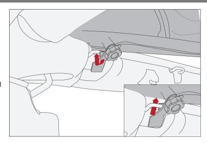
6. Tighten retainer arms by turning threaded lock knobs clockwise. Alternate between the left and right knobs to ensure tight fit.
