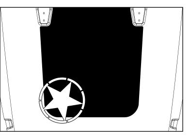
9. If any bubbles remain after transfer tape is removed, use the squeegee to remove them. Use the same center to outside motion as in step 7.
