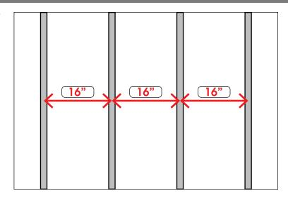
2. Determine appropriate mounting position. Using Lower Bracket for reference, mark and drill one  $1/4^{\prime\prime}$  pilot hole in the center of each stud. Pilot hole must go  $2^{\prime\prime}$  into stud.
