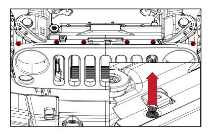
3. Pull bottom of grille away from vehicle to disengage metal clips on bottom rear of grille. Remove factory grille from vehicle.
