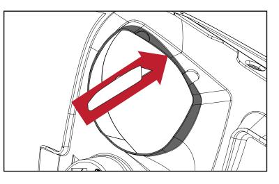
11. Install factory turn signal housing into Spartan Grille. Repeat for opposite side.
