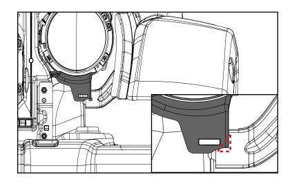
6. Remove ambient air temperature sensor from radiator support by pulling rectangular center pin. Move sensor and connected wires out of the way temporarily.
