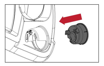
12. Install Spartan Grille using factory plastic retainers removed in step 2.
