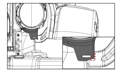
6. Remove ambient air temperature sensor from radiator support by pulling rectangular center pin. Move sensor and connected wires out of the way temporarily.
