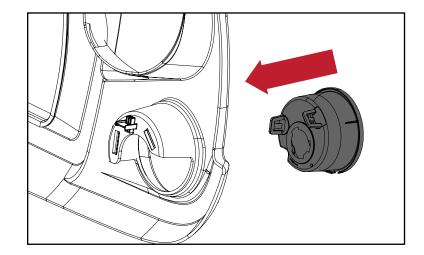
12. Install Spartan Grille using factory plastic retainers removed in step 2.
