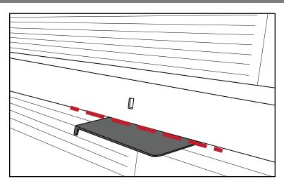
8. Flip sensor 180° from original position and reinstall using rectangular center pin.
