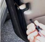
(2) Remove screws securing pull handle to door. Keep screws as they will be reused. Pull handle from door being careful not to dislodge threaded clip from inner mounting bracket.
