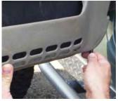
(4) Insert one end of new Nylon door strap through the front slot of the inner door skin. With hand Inserted into door from underneath align eyelets with threaded clip. Make sure not to dislodge clips. If this happens, simply reinsert and continue with installation. With handle ends installed push panel back and secure strap with screws saved in step (2).
