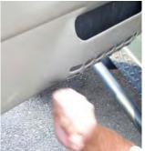
(5) Pop door panel back into place and reinstall screws removed in step (1). Repeat for other side.
