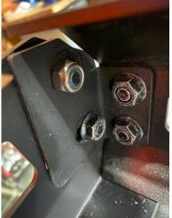
2. Slide the 3 center braces into place and attach with hardware. Use the longer button head bolts with 2 washers and Nyloc nut. Snug all the hardware but don't fully tighten at this time. With it only snug, it allows you to adjust the roof bracket when placing it on the Jeep later.
