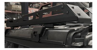
5. With the rack placed on the roof, slide the brackets to fit in the channel. Adjust as needed and measure to assure the rack is centered and square to the Jeep.
