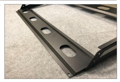
3. Slide the 5 center braces into place now attach with hardware. The first, middle and last center brace requires the longer button head bolt to pass through the center brace, rack and roof bracket. The second and forth center brace will use the shorter button head bolt to attach. Snug all the hardware but not fully tighten at this time. With it only snug it allows you to adjust the roof bracket when placing it on the Jeep later.
