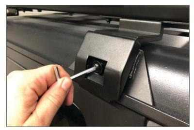
9. To complete the install fully tighten the roof bracket hardware.
