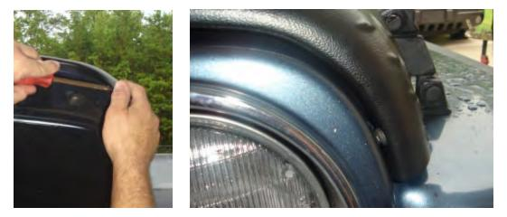
When properly installed the retaining screws should just be visible inside of the vehicle hood line and not interfere with the closing or locking of the hood.
