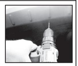
Step 64. Secure the flare to the wheel well using the supplied #8 screws. Do not over tighten screws.
