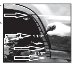
Step 34. Using a cutoff wheel or sawzall cut the lines made on the fender. Cut only the horizontal lines from inside of the fender to the vertical line drawn. Use caution when cutting. Do not over cut or cut into surrounding areas.
