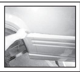
Step 42. Carefully cut the marked section with a sawzall or cutoff wheel. Use caution when trimming.
