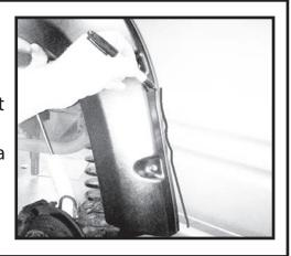
Step 40. Remove the retainer nut from the backside of the rear door that holds the lower body cladding on to the vehicle.
