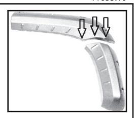
Step 50. Attach the rear and middle wheel arch flare sections using the supplied bolts and lock nuts with a washer on each side of the flare flange.
