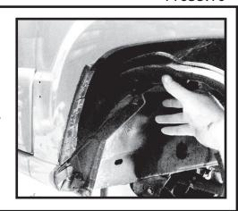
Step 18. Remove any and all emblems and lettering from the front fenders. Clean any adhesive from surface.
