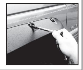
Step 24. Torque each bolt to 24 in-lbs (2 ft-lbs). Do not over tighten. Over tightening could cause damage or warpage.
