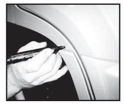
Step 31. Remove the section of trim from the front of the rear wheel well opening that is located next to the rear door edge.
