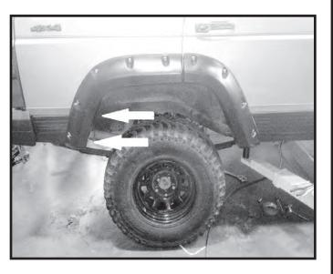
Step 41. Use of the trim tool may need to be used on any parts of the trim that have been misaligned during installation. To seat the trim against the body, the curved side will be used. To seat the trim side against the flare the flat side will be used. It may be necessary to start at one end and run the tool the full length of the flare.
