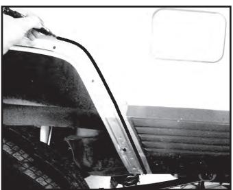
Step 33. Measure 3/8 inch up from the edge of the fender well and draw a horizontal line along the fender connecting the two lines made in the previous steps. Repeat for opposite side.
