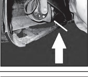
Step 16. Bare metal must be treated. A primer surfacer is recommend before painting.
