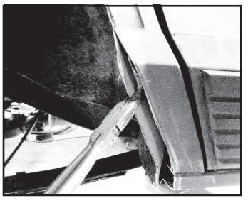
Step 38. Install the dog leg shaped trim piece on the door edge. At the rear door opening fit the trim against the body. Secure the trim in place with the supplied self tapping screws. Use the dimples in the plastic as guides for the screws. Do not overtighten. Repeat for opposite side.
