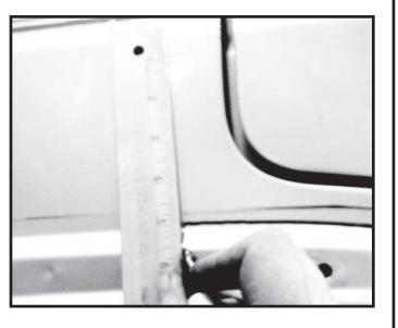
Step 32. At the bottom of the rear portion of the wheel well housing measure a distance of 1 5/8 inch from the the wheel well towards the rear of the vehicle.
