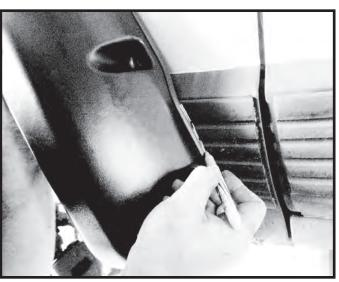
Step 21. Using a putty knife lift the body trim off of the body enough to cut with a razor knife.
