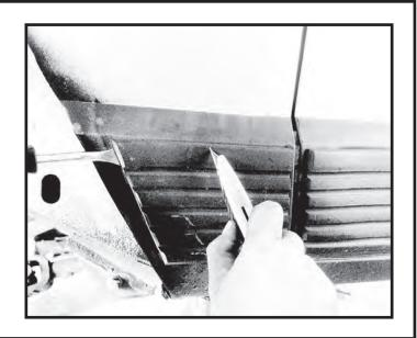
Step 22. Once fitment is complete hold the flares in place and mark the mounting holes on the body using the pre-drilled holes in the flare as a guide.
