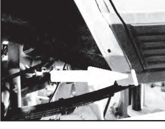
Step 30. Starting at the mark made in the previous step continue following the contour up maintaing a 2 inch distance from the wheel well. The line shall continue to 1 inch past the door opening. Repeat for opposite side.
