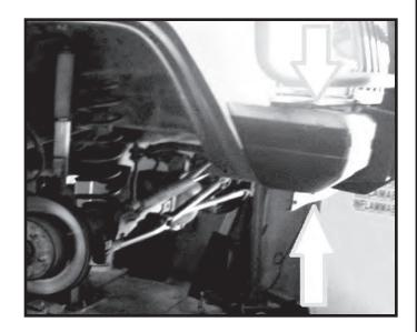
Step 3. Unbolt the front airdam from the supports on each front lower section of the fender. The supports will be cut out in later steps.
