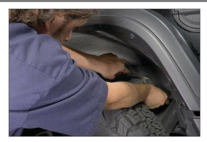
2. With the inner liner loose now you can remove the entire fender. Grab the fender and pull the fender away from the body. It's attached with clips. When pulling it away the clips will probably break but its okay your not reusing them. Start pulling from one corner and work your way to the other side of the fender.
