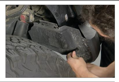
5. Remove the plastic shield from the bumper. It also has three M8 bolts attaching it.
