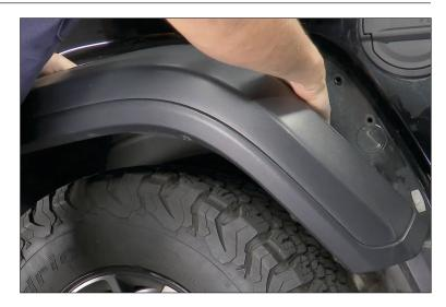
3. With the OE fender and liner removed clean the body of the Jeep in this area. This area retains mud and dust. If you see any scratches or paint is rubbed away, prep and paint areas to assist in rust prevention.
