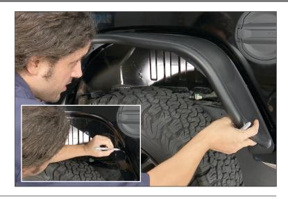
8. There is NO drilling necessary for this install. The nutserts will fit into the factory holes you marked in the previous step. To properly install we highly recommend using a nutsert tool. Insert nutserts into the Jeep body using the tool to crush the nutsert to the body. Take your time and assure each nutsert is crimped fully to avoid it from spinning or
