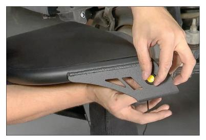
12. Clean the sheet metal of the Jeep where the steel fender will meet. Place fender into place to the vehicle. The brackets will support the weight of the fender.
