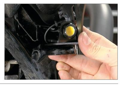
15. Concerning the method of wiring use your preferred method. We selected wire splices with heat shrink ends. We would also recommend soldering and using heat shrink as the best method of connection and keeping the connections waterproof.
