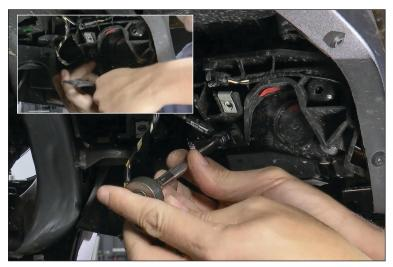
6. Disconnect side marker lights and front running lights. There are some zip ties that will need to be snipped to release the harness from the fender.
