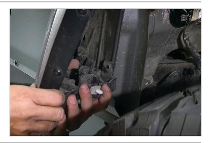
3. Unplug the fender wiring from the chassis harness
