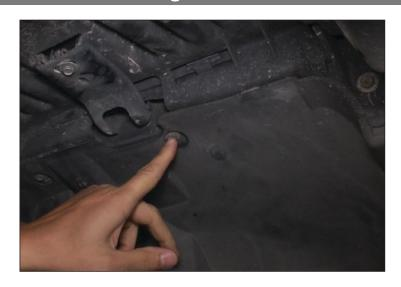
2. Remove body clips that attach the inner fender to the body. Use special removal tool to pry out.
