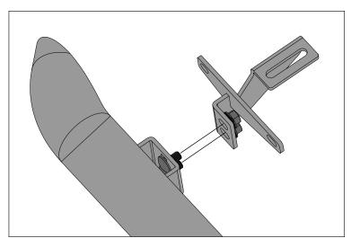
3. Starting with the passenger side, carefully raise the Mounting Bracket up to the pinch weld of the body and align the pinch weld tabs with the 6mm mounting holes. Loosely install the (4) Short M8 Hex Head and Flange Nuts.
