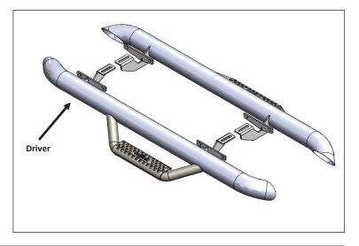
2. Using M10 Carriage Bolt and M10 Flanged Nut, loosely attached mounting brackets to Nerf-step.
