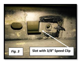
**Step. 4** Starting with the passenger side, carefully raise the bar up to the pinch weld of the body and align the pinch weld tabs with the 6mm mounting holes. Loosely install the (6) M6 x 20mm Hex bolts, washers & nuts. Do NOT fasten down tightly, as you may need to lightly adjust the bar upon applying remaining locations. Note: Some models may require drilling out additional 6mm mounting holes in each pinch weld tab location.
