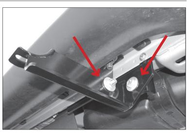
19. Bolt Rear Inner Support Bracket to back of Mounting Bracket with 10mm x 30mm Hex Bolt, 10mm Flat Washers, and 10mm Nylon Lock Nut. Do not fully tighten.
