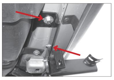
18. Line up hole in Outer Support Bracket with hole in Mounting Bracket. Bolt Brackets together with 10mm x 30mm Hex Bolt, 10mm Flat Washers, 10mm Lock Washer, and 10mm Hex Nut.
