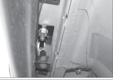
4. Next, select the Driver Side Front Mounting Bracket. Bolt Front Mounting Bracket to back of pinch weld with 6mm x 25mm Hex Bolts, 6mm Flat Washers, and 6mm Nylon Lock Nuts. Do not fully tighten.
