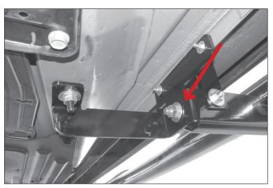
8. Line up hole in Outer Support Bracket with hole in Front Mounting Bracket.
