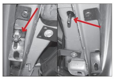
**NOTICE** Outer Support Bracket will line up on rear facing side of Mounting Bracket
