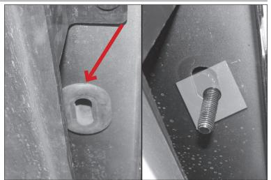
5. Attach Mounting Bracket to Bolt Plate at pinch weld with 12mm Flat Washer, 12mm Flange Nut, 6mm x 25mm Hex Bolt, 6mm Flat Washer, and 6mm Nylon Lock Nut (Figures 6 & 7).
