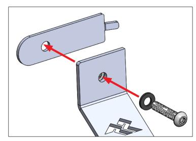
2. Place a M10 carriage bolt through each bracket. Then place the rubber isolator over the carriage bolt threads. Now position your off-road jack over the carriage bolt then install the M10 washer and thread the hand knob to the carriage bolt.
