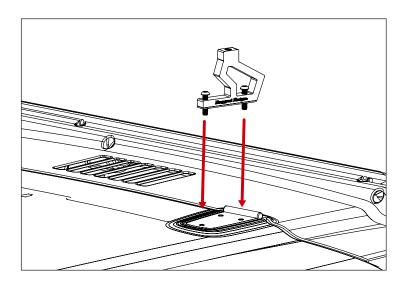
3. Align Offraod Jack slotted holes to Hood Brackets and affix using supplied Thumb Screws.
