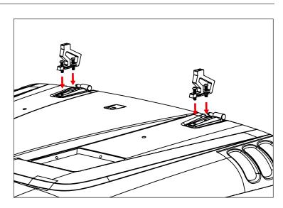
3. Align Offraod Jack slotted holes to Hood Brackets and affix using supplied Thumb Screws.
