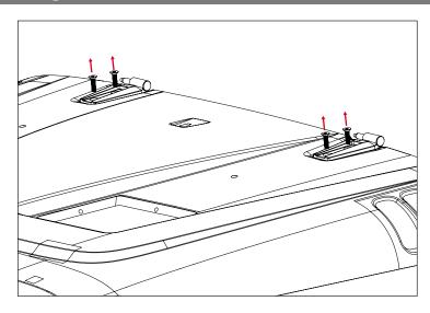
2. Loosely attach Hood Brackets to hood hinge using supplied M8 button head bolts.
