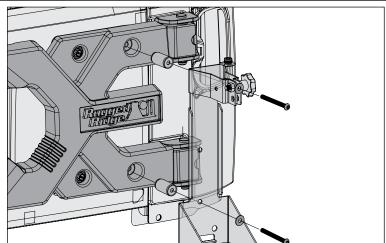
3. To install Off Road Jack, use bottom knob to clamp base of jack into position ensuring rear of base is under tab in mounting bracket. Close top swing arm making sure rubber pads grip jack's vertical beam.
