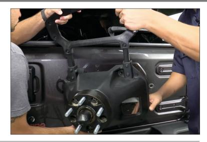
2. Attach Spare Tire Relocation Bracket to tailgate using the OE hardware just removed. Tighten in an alternating pattern. **Avoid using power or air tools**. Tighten to 20ft lbs torque.
