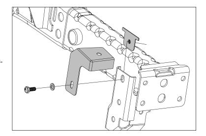
8. Position Bumper Shell and Tow Hooks into place on vehicle's frame rails. Using supplied M12 hardware and Nut Plates, loosely attach Bumper Shell and Tow Hooks using center four holes.
