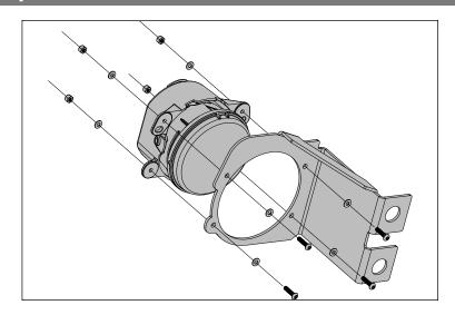
3. Using supplied M10 hardware, loosely attach Winch Tray Bracket to Winch Tray.
