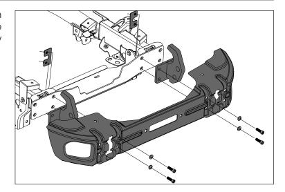
8. Loosely attach Light Bracket using supplied M12 hardware.
