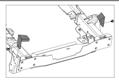
7. Position Bumper Shell and Tow Hooks into place on vehicle's frame rails. Using supplied M12 hardware and Nut Plates, loosely attach Bumper Shell and Tow Hooks using center four holes.
