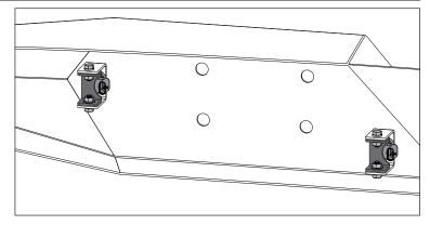
3. Insert M14 Nut Plate in passenger side frame opening and loosely install Mounting Brackets using supplied M14 hardware.
