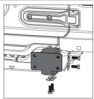
4. Install Bumper and D-Shackle Tabs using supplied M12 hardware. Once bumper is in position, fully tighten Mounting Bracket hardware.
