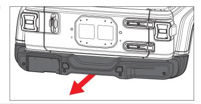
2. Install factory back up sensors (if equipped) or supplied Rubber Plug in Spartan Rear Bumper using M6 hardware and Sensor Brackets.
