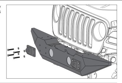
6. Fasten Spartan Front Bumper to Winch Plate using supplied M8 hardware. Tighten all fasteners and reconnect fog lights.
