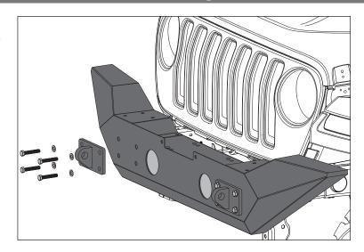
6. Fasten Spartan Front Bumper to Winch Plate using supplied M8 hardware. Tighten all fasteners and reconnect fog lights.
