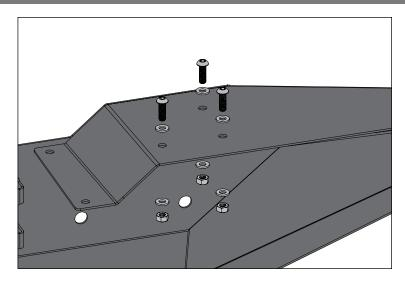
2. Install Spartan Overrider using supplied M8 Nut Plates and removed M8 Bolts and Flat Washers.
