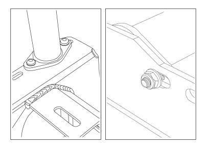
3. Loosely tighten this hardware. The bars should be able to slide on the center base, so DO NOT full tighten at this time. Attach all three bars then set the assembly aside.
