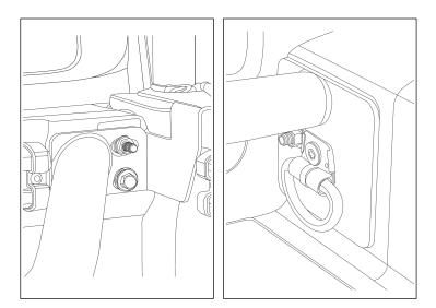
9. Install the adjustable tire mount to the mounting base. Pass a M12 bolt through a M12 washer, through the top slot on the mounting base from the outside surface. Then, from the inside surface of the mounting base, install a M12 washer over the bolt and thread on a M12 nut. Repeat this process at the left and right slots. With the hardware loose adjust the tire mount to the desired height. Check this to the backspacing of the tire you plan to mount, then, fully tighten the M12 hardware.
