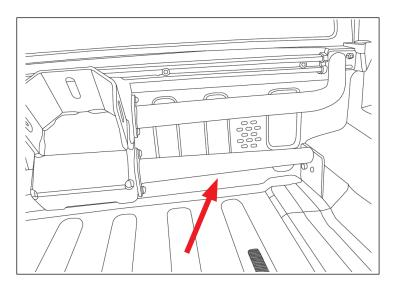
8. At the upper location on both the left and right sides, install the M8 Button Head Bolt into the threaded hole. At the lower location on both the left and right sides, reinstall the tie down into the threaded hole.
