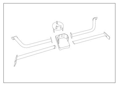
2. Using M8 hardware attach the bars to the center mounting base. Notice the M8 hardware button head has a black finish. Use the black flat washer exposed on the outside and use the M8 zinc flat washer and zinc nylock nut on the inside.
