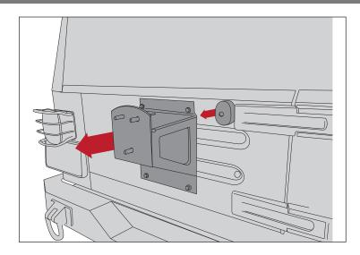
5. Remove stock tailgate hinge plastic covers. Remove stock tailgate hinges.
